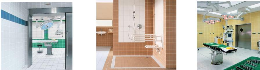
By means of the photocatalysis, activated oxygen is produced which decomposes micro-organisms such as bacteria and fungi, but also algae, moss and germs without any chemical products and prevents their renewed formation - a convincing advantage for example in medical areas like operating theatres.
